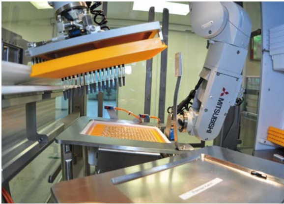
Picture 5: The solution can supply syringes to the discharge track at a rate of 400 per minute. Other products on the market take up three to four times more space compared to the compact MRT cell.
