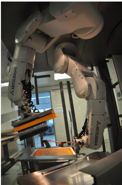
Picture 6: Robots bring flexibility and efficiency to production. In the pharmaceutical and medical technology sectors, they are increasingly taking on handling tasks to reduce human effort, for example by supplying filled syringes to the end-of-line packaging station.
