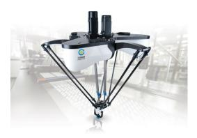
**Picture 1:** The high speed Codian Robotics pick-and-place solution is built on Mitsubishi Electric proven servo technology that integrates seamlessly with a Mitsubishi Electric controller for fast integration and reliable operation.
