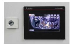
**Picture 5:** The SCM analysis from Mitsubishi Electric provides detailed diagnostics, offers suggestions for where additional measurements should be taken, and provides maintenance staff with more precise error identification.
